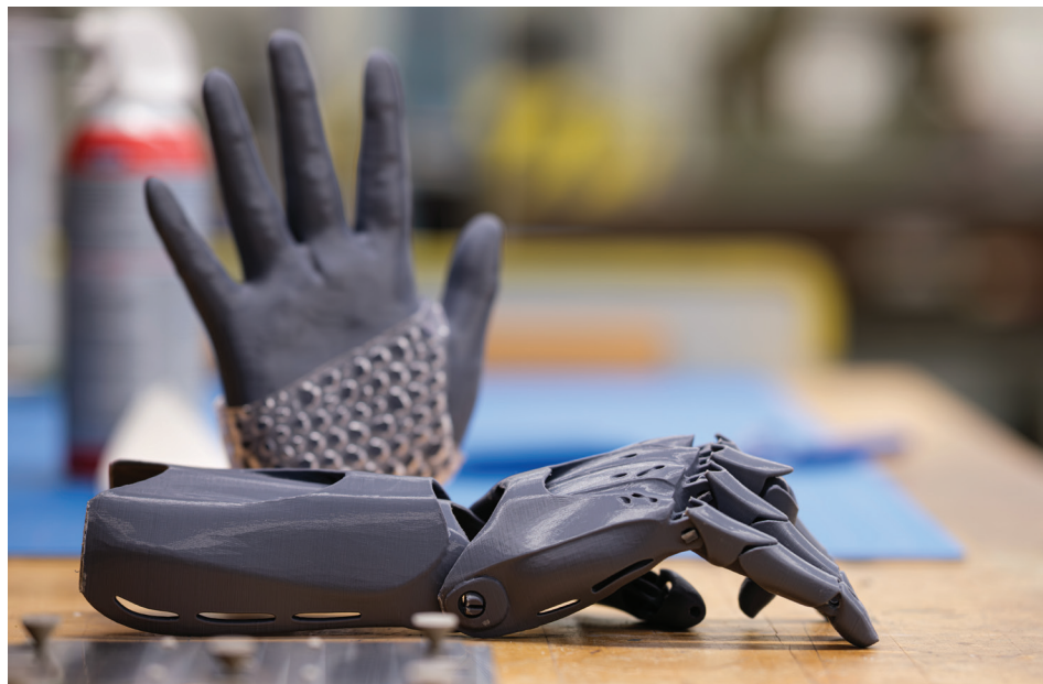
Handiwork. A 3D-printed wrist-actuated prosthetic hand (front); and a 3D print of an individual’s hand with a second print of webbing (back) as a custom brace/cast design to demonstrate a perfect fit that can go, well, hand in glove.
