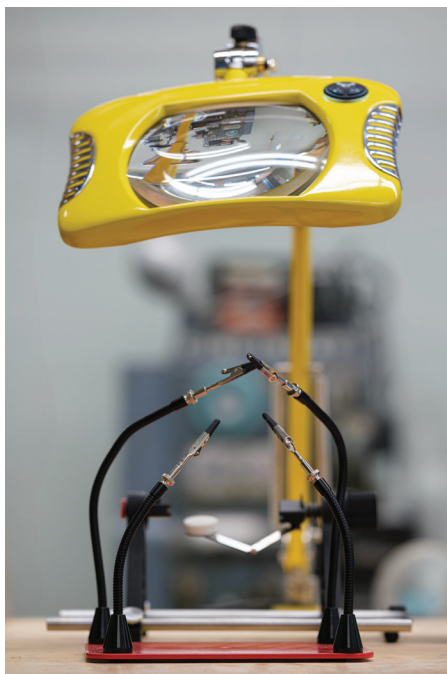
Not Pixar but it is a 'helping hands' soldering station with magnifying lamp.
