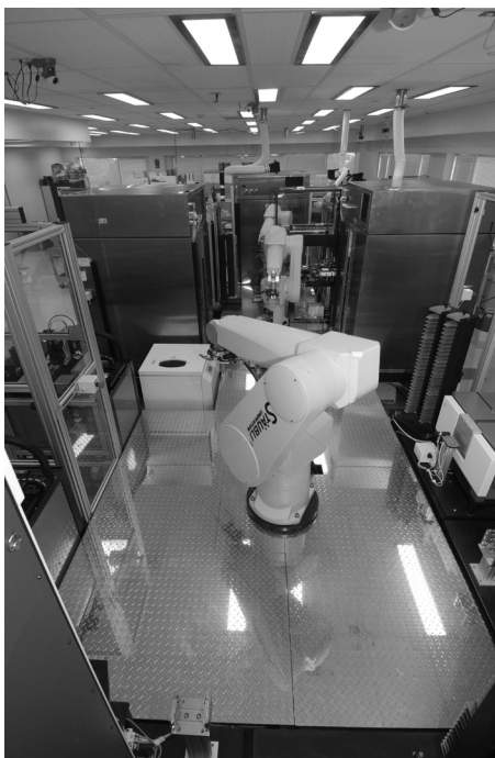
Kalypso robots at the NIH Chemical Genomics Center used for plate handling, which will help scientists profile more than 100 P. falciparum malaria field strains. Credit: Maggie Bartlett, NHGRI.
