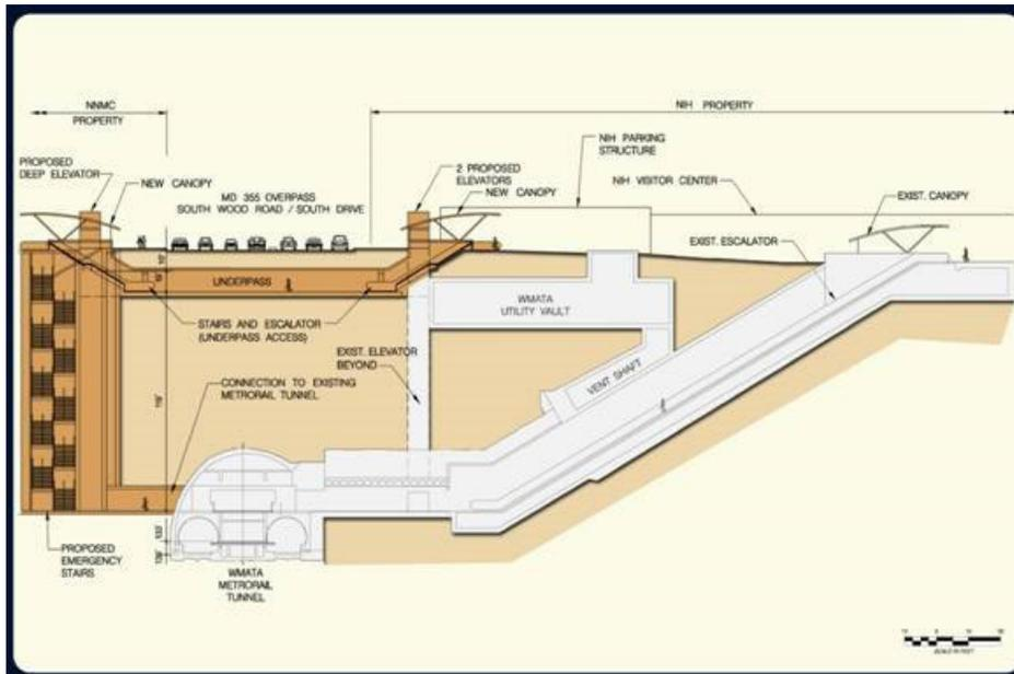
A pedestrian tunnel under Rockville Pike near the South Drive intersection would allow for safer pedestrian access between Walter Reed National Military Medical Center and NIH. The Medical Center Metro Crossing Project also includes a new high-speed elevator from the Metro station to the east side of the roadway and an emergency egress stairwell.
