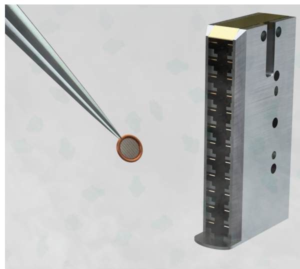
Carbon grid with frozen protein sample prepared for loading into cryo-electron microscope cartridge.
