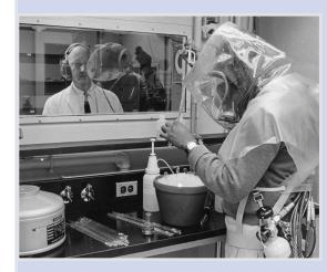
This oxygen-free, steel-framed box was the first of its kind to be used for biomedical research. Built in 1967 for \$250,000, NIH's anaerobic laboratory was primarily used by Earl and Thressa Stadtman's groups to work with certain enzymes and other biological compounds that are inactivated when exposed to oxygen. The room was filled with a mixture of nitrogen and hydrogen and contained a variety of instruments. Anyone working in the room had to wear a
