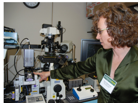
NHLBI biologist Clare Waterman can view the protein building process live using nanotech tools like this homemade total internal reflection fluorescence (TIRF) apparatus.
