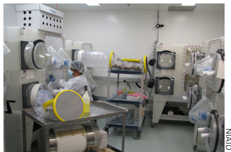
In NIAID's gnotobiotic mice facility, technicians handle the germ-free animals with gloves attached to isolators.
