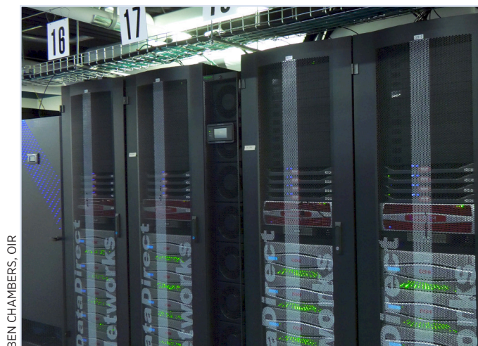
Combined, Biowulf's 10 high-performance storage systems, two of which are pictured here (each occupies two racks), provide more than 25 petabytes of storage capacity.
