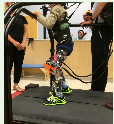
A child with cerebral palsy, assisted by the NIH pediatric exoskeleton, walks across a surface.
